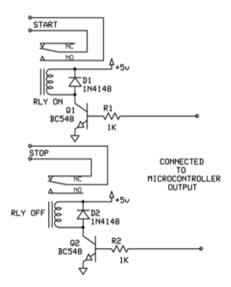
The above figure and circuit shows the relay driver circuit, which we are use to start and stop the motor or motor starter.
