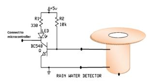
Rain water detector means we will detect the presence of rain i.e. without being present at that site we will be able to know the condition of rainfall whether it is present or absent. So that the farmer will be able to know about rainfall on his mobile and will take proper action that is whether to give water to the crops and turn ON or OFF the motor.
