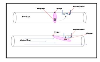
For the safety of motor pump it will check motor is running without water, which causes motor damage or burn.
