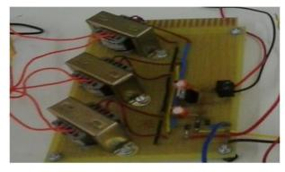
In this we used three transformers of range 230V AC 0-9V/0.25A, which are connected to three phase of supply board and this is the power supply which gives constant 5V regulated power supply and also gives three phase supply to the circuit.
